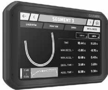
Example of post-session analysis on the full-color Catalyst screen, comparing two lines through a corner. In this example, time spent in the corner, peak acceleration/braking, and time spent accelerating and braking are being compared both graphically and numerically.
